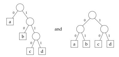
correspond to  $C_1$  and  $C_2$ . The code word for a given symbol can be obtained as follows: Start at the root and descend toward the leaf node associated with
