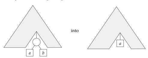
The frequency of a in the result is the sum of the original frequencies of a and b, so as not to alter the tree's weight.
